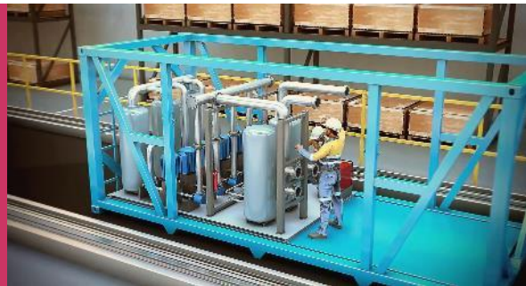
Factory built, tested and commissioned (and transported)**
