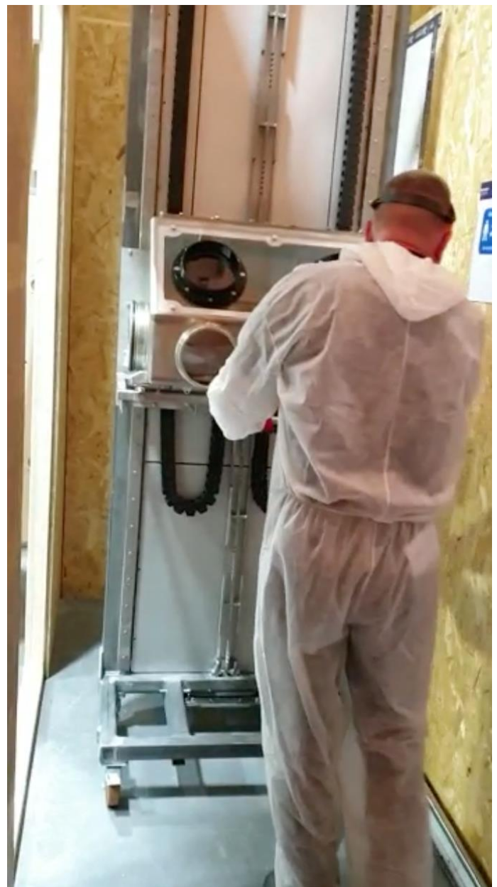
Pictured: An operator using the specially designed inerting box on a test rig
